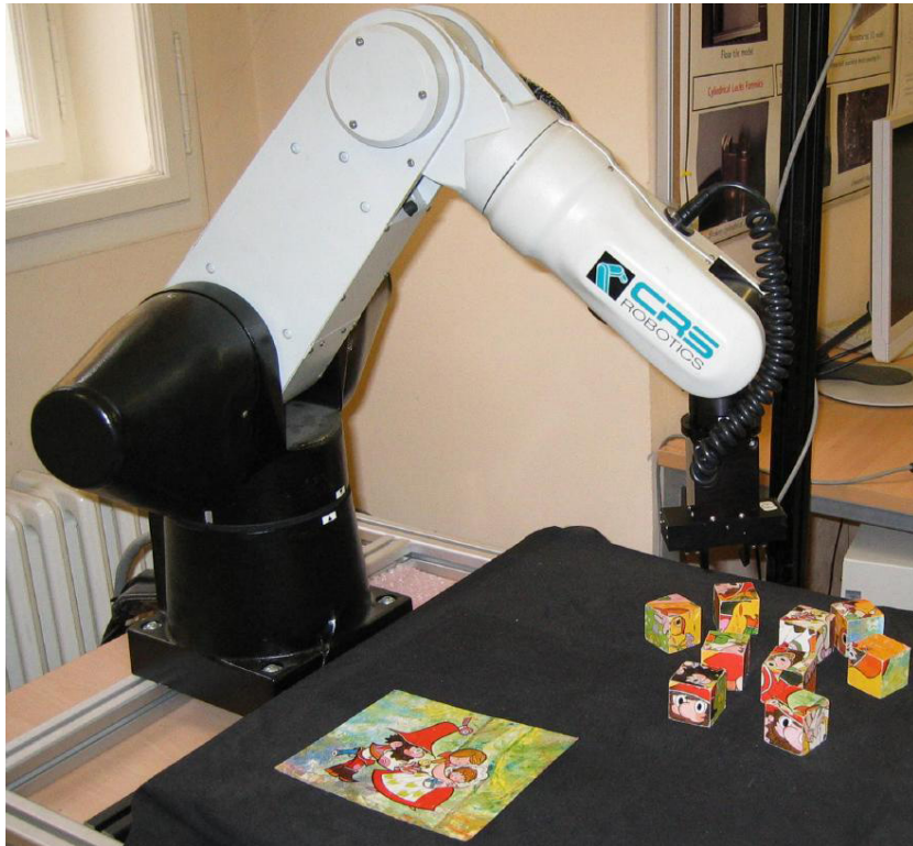
Figure 7.1: COSPAL project related task - cognitive robot puts the cubes together.
