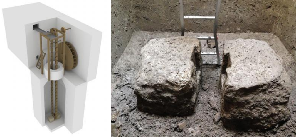
Figure 5 Reconstruction of the water-lifting technology from the cistern v and photographic documentation of the architectonic evidence (author: J. Sou ek).
