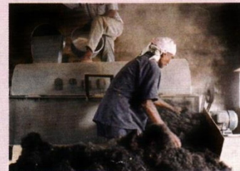
This human hair is waste from a wig-making factory. It will be processed into L-cysteine for use in food and medicines using enzymatic hydrolysis.
