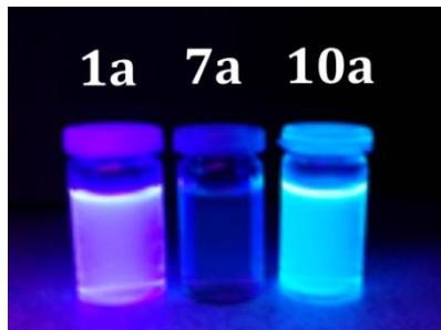
**Figure 2** Starting deazapurine **1a** aminated product **7a** and 8-(methylamino)-7-deazapurine **10a** in methanol under UV-light (366 nm).
