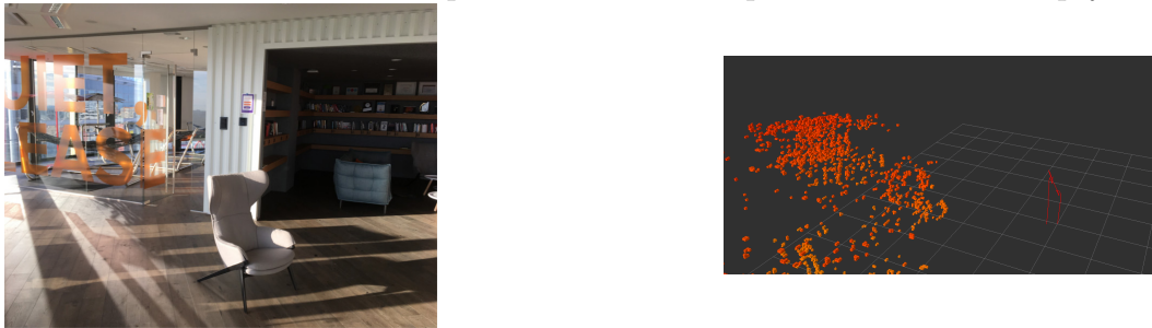
Figure 8.1.3: A comparison between the photograph of a scene with a chair and the octomap representation of the scene with the chair. The chair is also clearly detectable by our perception system.
