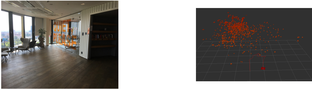
Figure 8.1.1: A photograph of a room used to conclude obstacle perception experiments and the octomap representation of that room, created by the system's current implementation.
