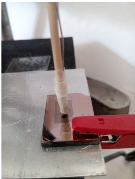
Fig. 2-5 GNFE with pNIPAAAM substrate connected to the potentiostat with reference gel leakless Ag/AgCl electrode and platinum wire as an auxiliary electrode.
