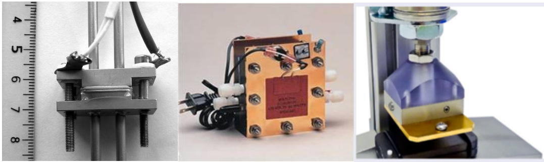
Figure 2.5.2: Fuel cell testing hardware. Left: Old laboratory-made design, 1cm 2 electrode area, stainless steel. Middle: commercial cell 1 cm 2 (Electrochem.org), graphite plates. Right: modern cell with 5cm 2 active area (TP-5, Greenlight Innovation), graphite plates. Designed for fast assembly/disassembly, pneumatic compression holder allows quick and easy exchange of cell.
