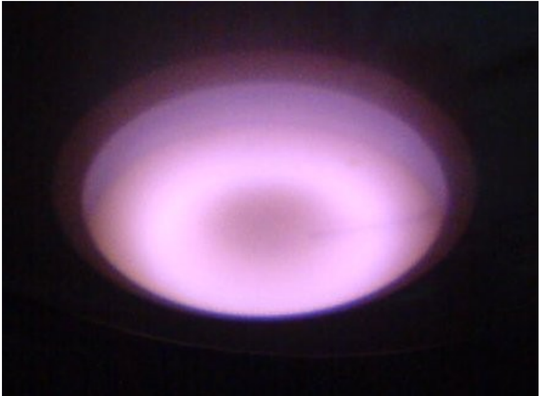
Figure 2.1.2: Photography of magnetron plasma discharge in argon during operation. Note the wire on right side made of platinum, forming composite target with CeO_2 . This is one of the possible configurations that can be used to prepare sputtered Pt-CeOx mixed oxide
