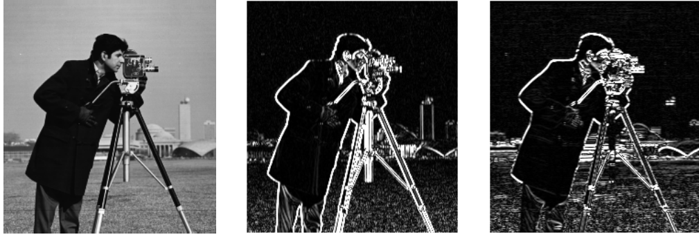
Figure 6.1 An image and its derivation in x (horizontal) and y (vertical) axis.
