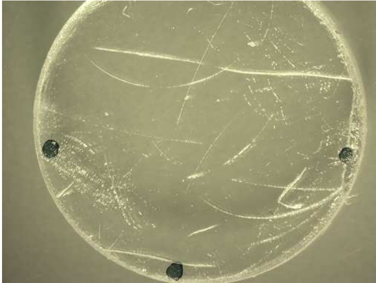
Figure 35: Surface image of sample 2S9, magnification 8x taken with optical microscope. Tb:YSO films grown on Ce:YSO \langle 010 \rangle substrate from the PbO flux., with defects (shown pit aggregation along substrate defects, looking like scratches, induced during polishing)
