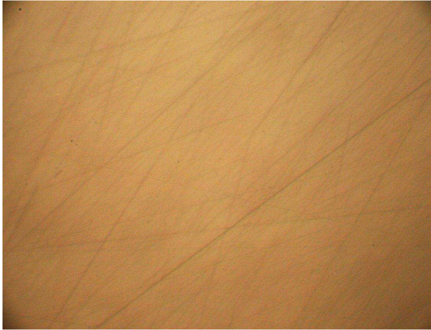
Figure 34: Microscope photography of the LuAG substrate oriented at \langle 111 \rangle , etched in sulphuric acid ( \text{H}_2\text{SO}_4 ) and phosphoric acid ( \text{H}_3\text{PO}_4 ), magnification 12.5x. Revealed deep defects in form of scratches, induced during the polishing stage by grains of polishing media.
