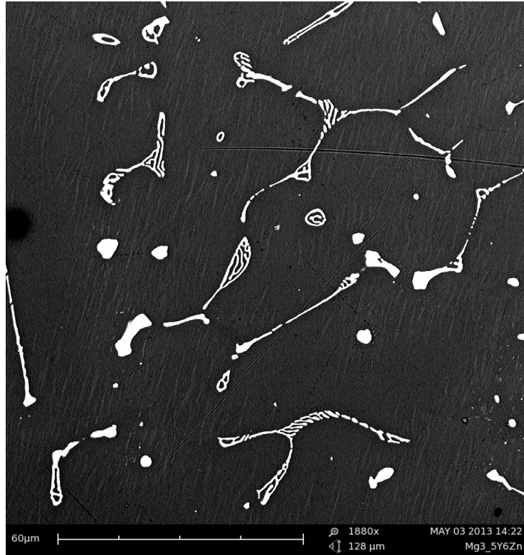
Figure 5.7: SEM image of as-cast Mg 3 Y 6 Zn alloy, detail.
