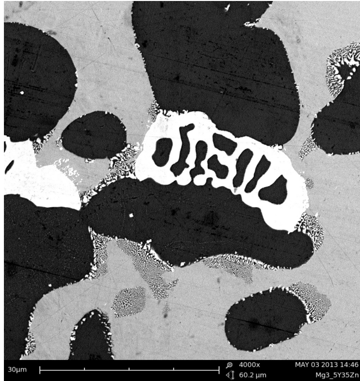
Figure 5.11: SEM image of as-cast Mg 4 Y 26 Zn alloy, detail.
