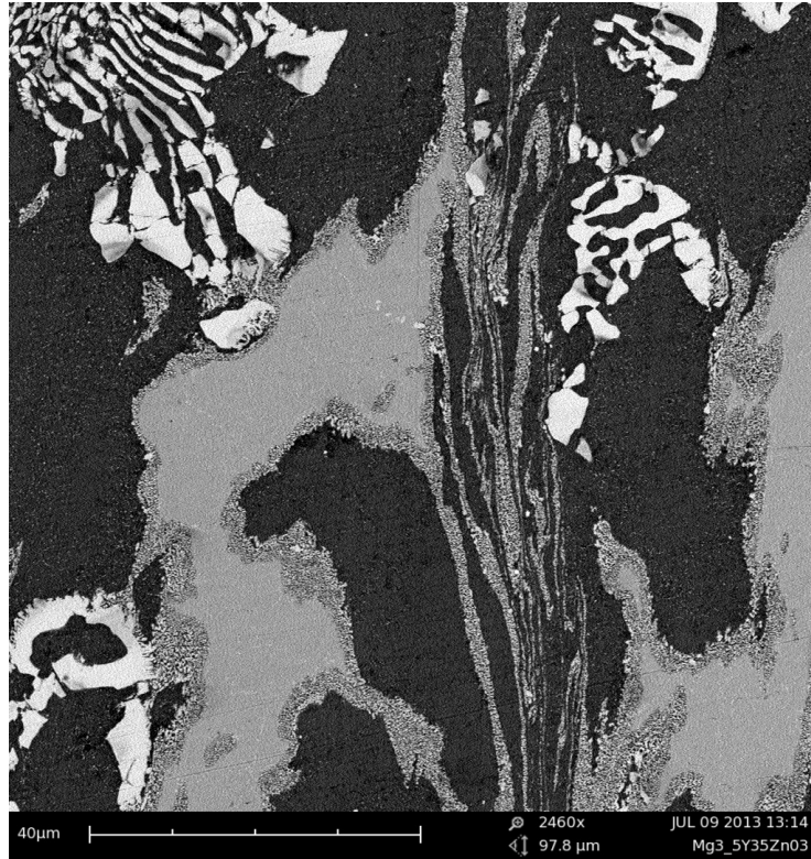
Figure 5.64: SEM image of Mg4Y26ZnE200 sample after 4 passes, the normal direction. A detail showing ductility of Mg-Zn phases in the zone of localized deformation.
