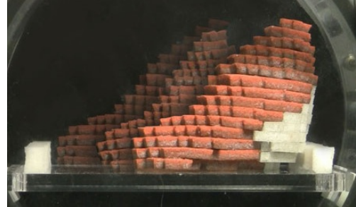
(c) Prototype of a physically constructed voxel-based robot actuated by changing air pressure [27].
