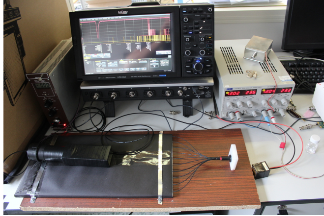
Figure 6.3: Photo of the whole measuring system. Testing holder, plate, PMT, digital oscilloscope, and high voltage.
