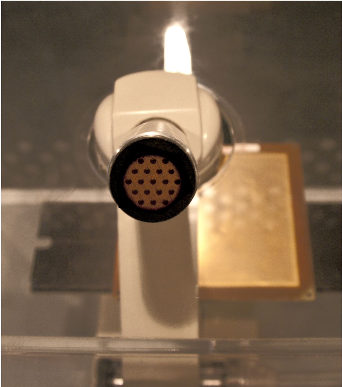
Figure 3.3: A sample of GEM plate placed under a microscope in CERN Microcosm exposition to show the scale of the holes etched in the Kapton foil.
