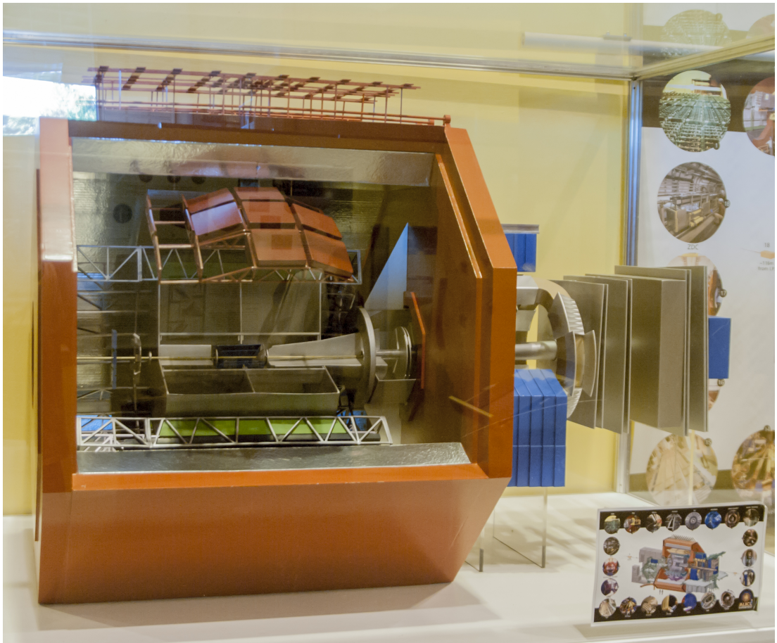
Figure 2.4: A model of ALICE experiment with the cherenkov counter visible in the top section as seven red blocks inside the red casing of the detector.
