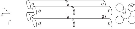
FIG. 1. The geometry and dimensions of the trap. The origin of coordinates is situated in the center of the trap.
