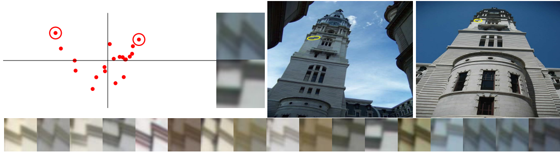
Figure 3.7: A 2D PCA projection of a feature track of SIFT descriptors (left); the most distant patches and their images (right); sample of feature patches from the track. The distance of the most distant SIFT descriptors is 593 and is caused by the viewpoint and scale change.
