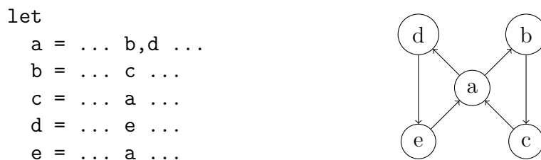
Figure 2.1: Illustration of loop-breaking a recursive definition. Set \{a\} certainly a loop breaker, but so are the sets \{b, d\} or \{c, d, e\} .
