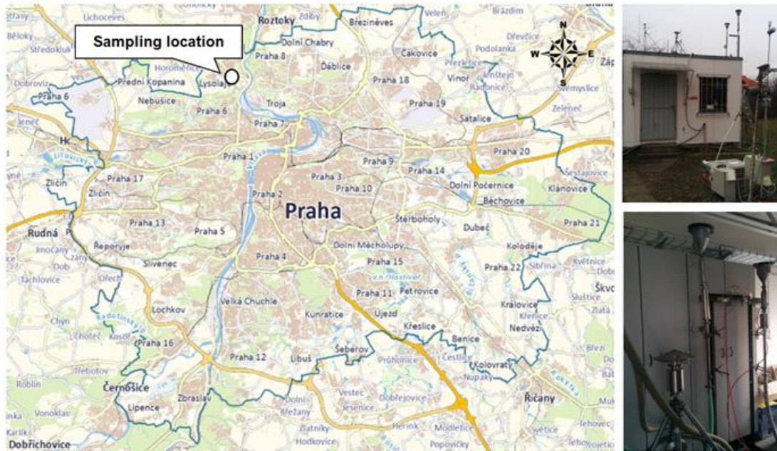
Figure S1. Sampling location in Prague and impactors deployed in outdoor (top right) and indoor environment (bottom right) (IPR, 2015).
