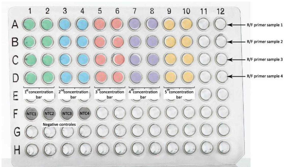
Fig. 9: Schematic design of positions of samples for efficiency determination with real-time PCR. Each color represents a certain concentration. In the 1 st concentration bar is the highest concentration – 1000 relative units, 2 nd – 200, 3 rd – 40, 4 th – 8 and in the 5 th was 1.6 relative units. Each line (labeled A, B, C, D) contained a verified R/F primer. NTC – no template control.
