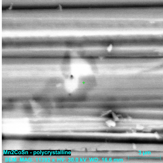
Figure 3.1: An inclusion seen by EDX. The measurement under the green cross shows weight percents 44.90% (Mn), 12.88% (Co) and 42.27% (Sn), which correspond to the normalized composition (see Table 3.1) 2:0.53:0.87.
