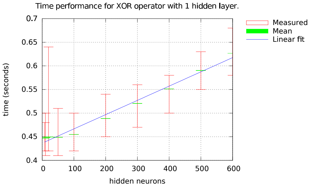
Figure 4.1: The time results of the MLP network solving XOR with a variable number of neurons in one hidden layer. The resulting values are averaged over 100 runs. The test was run on the development machine using GPU for parallel computations.
