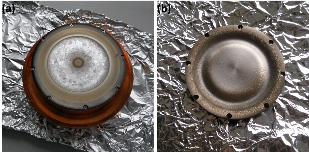
Figure 2.6: (a) Mg target used for deposition of Mg films studied in this work. (b) Al target with a very clearly visible erosive zone. Both targets are 100 mm wide in diameter
