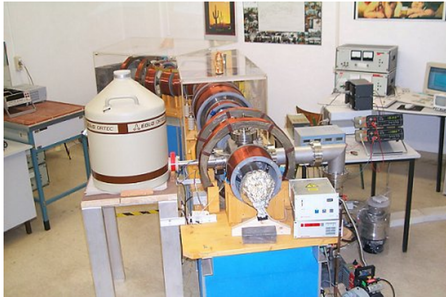
Figure 4.7: A picture of the laboratory in HZDR and the slow positron beam SPONSOR.
