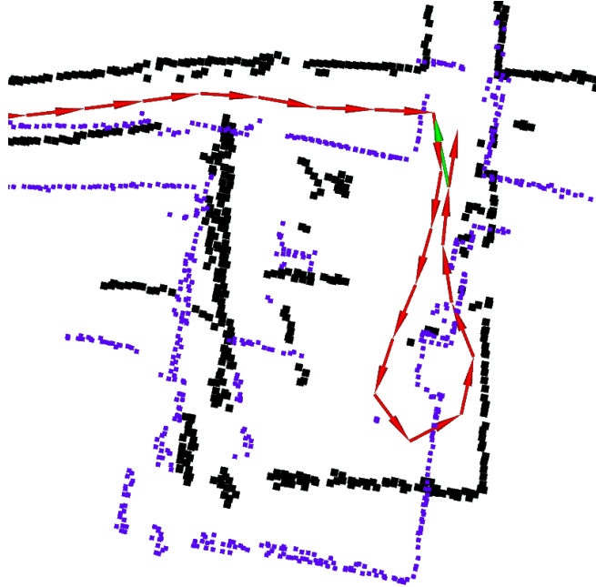
Figure 3.2: Picture shows a difference between moving window in purple and NDT map corrected with loop closures in a white color.
