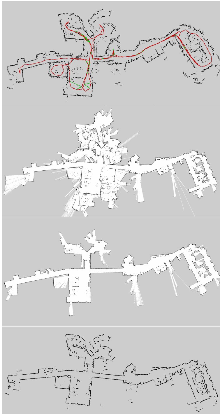
Figure 5.5: Map of the corridors mapped by our NDT approach, Hector Mapper and Gmapping. Visualization of our approach includes visualization of pose graph with red odometric edges and green loop closure edges. White spots represent means of each cell's normal distribution. The last picture represents the ground truth.
