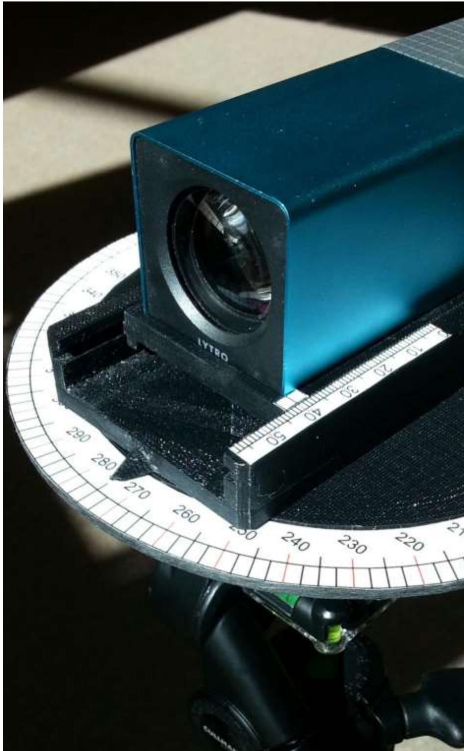
Figure 47. A Lytro camera mounted on panoramic tripod head designed and 3D printed at Johannes Kepler University, with permission. Source: [2]
