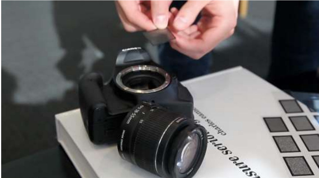
Figure 16. A printed coded mask being applied to a standard Canon camera. Photo courtesy by Kshitij Marwah, with permission.
