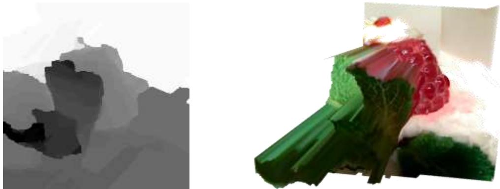
Figure 33. 2D depth map (left) and spatial data mapped to 3D (right), a raspberry cake, photo by author. Rendered by software accompanying the thesis.
