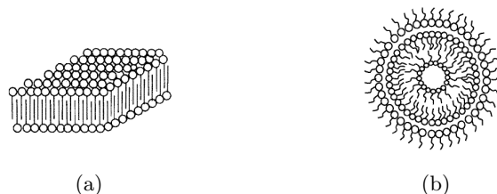
Figure 3.6: Schema of lamellar (a) and onionlike (b) structures formed by surfactant molecules in solution;Ganguli et al. (2010).
