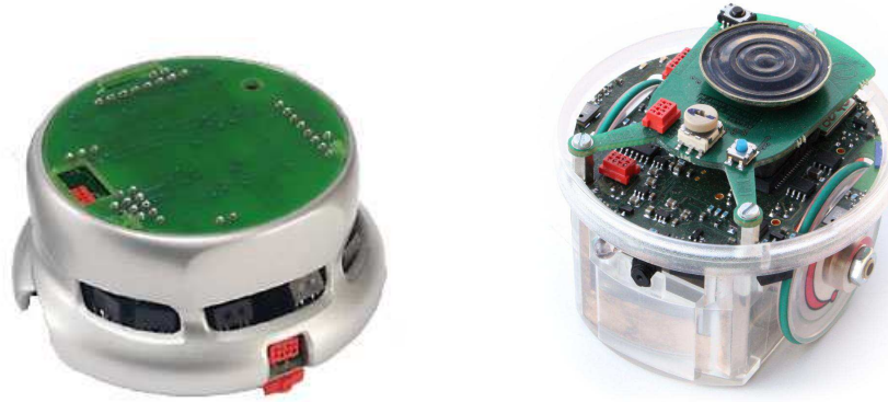
Figure 1.4: Left: The first widely used miniature robot Khepera built by K-Team SA ( www.k-team.com ). Right: Follower of Khepera robot named E-puck.
