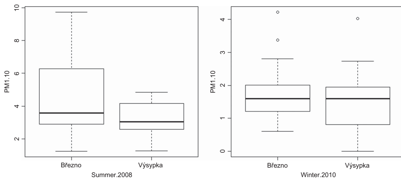
Figure 2. Box-and-whisker plots for PM 1–10 mass concentration at sampling sites Březno and Výsypka in summer and winter seasons.
