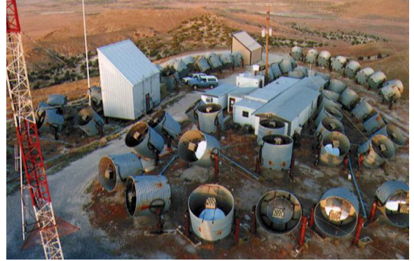
Figure 2.6: 67 detectors containing 880 photomultipliers in total at Little Granite Mountain. Barrels are set to positions which ensure full sky coverage of all modules.
