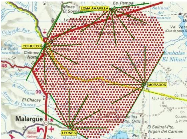
Figure 3.1: The detector layout of the Pierre Auger Observatory. Red dots indicate SD stations which are overviewed by 4 FD buildings. There are 6 fluorescence telescopes in each building. Green lines indicate field of view of each telescope.
