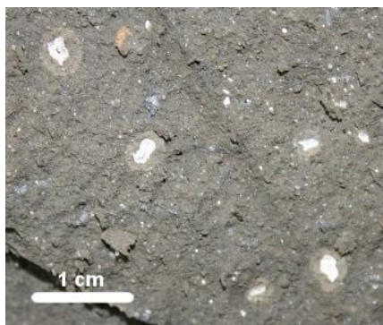
Fig. 2 Newly formed gypsum with illitic aureole in the backfill of the Mock-Up-CZ experiment.
