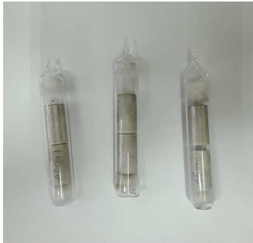
Figure 3.2: Quartz ampules after centrifugation containing the crucibles with crystals and residual flux.
