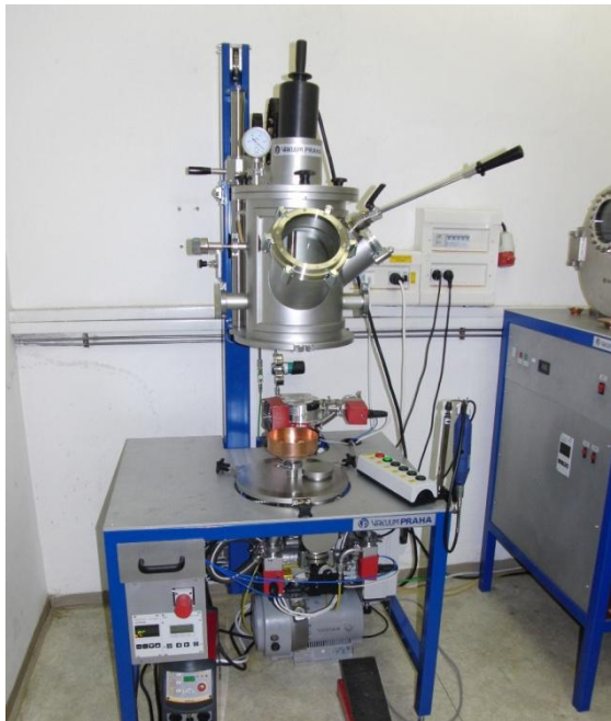
Figure.5.1. Photo of mono-arc furnace used for melting of initial components
