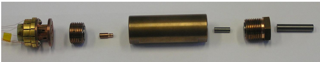
Fig. 2.6: A pressure cell designed for not only electrical resistivity measurements. From the left to the right: a reduction for connection with PPMS instruments, a plug support, a plug, the body of the cell, a piston, a piston support, and a pushing rod used during changing pressure inside the cell.
