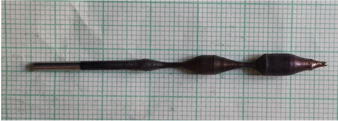
Fig. 3.2: An ingot obtained from the growth #10 by Czochralski method. On the left end there is a tungsten holder serving as the starting seed. During this preparation two necking parts were made.
