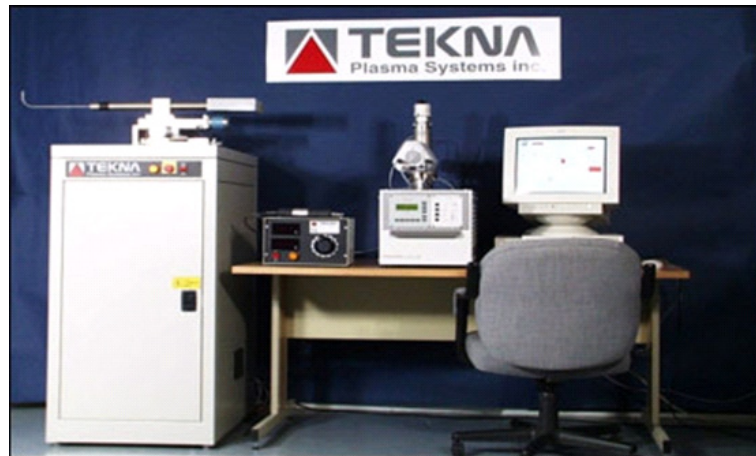
Figure 3.12 The enthalpy probe system of Tekna Plasma Systems Inc.
