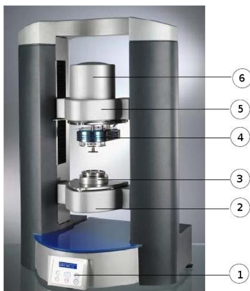
Figure 4.5: Haake Mars III - 1. Display and control panel, 2. Holder for tempering units, 3. Electric temperature-module TM-EL-P, 4. Electric temperature-module TM-EL-H, 5. Holder for measuring head, 6. Measuring head; (see the Instruction Manual Haake Mars III , Thermo Scientific, Ver. 1.5, p. 40)
