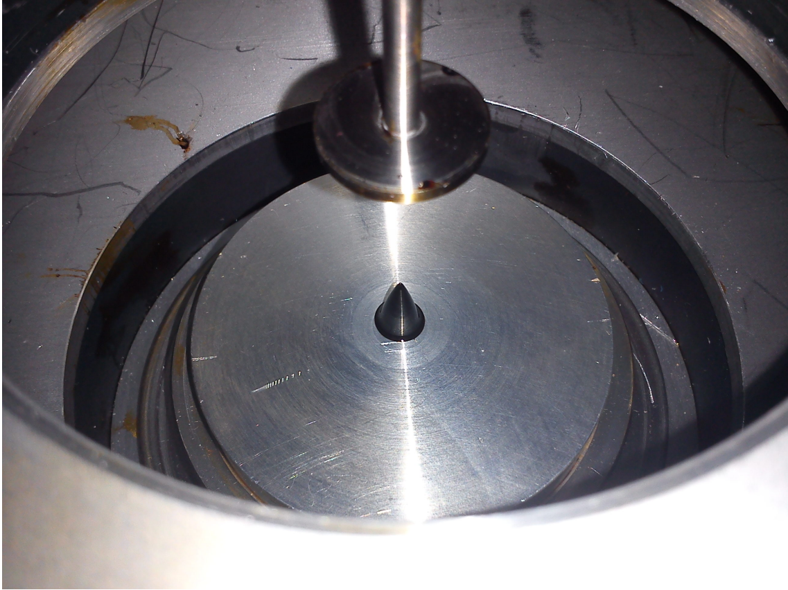
Figure 5.33: Sample of ferrofluid APG513a OLD - one droplet in a homogeneous magnetic field (an example of Rosensweig instability)
