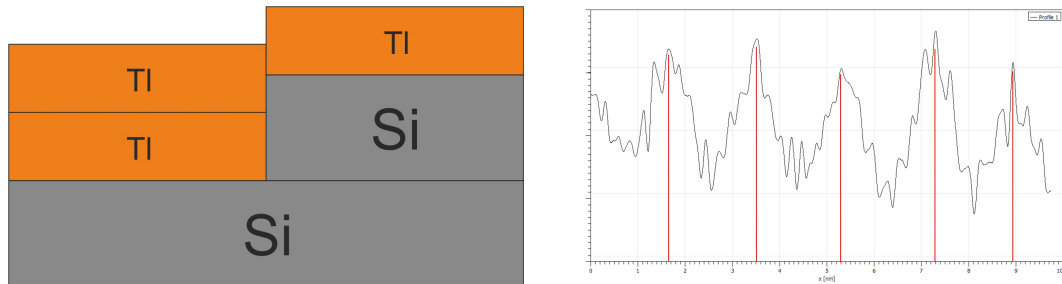
Figure 5.4: The second layer of Tl in the proximity of the step edge of the terrace.
