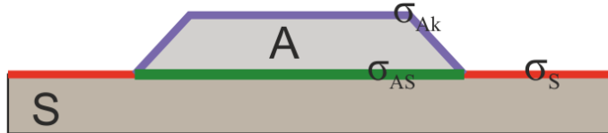
Figure 2.3: Energy balance of the surface growth in the 2D mode: S - substrate, A - adsorbate \sigma_S - density of the substrate's free surface energy, \sigma_{Ak} - surface density of the free energy of the k^{th} type of the adsorbate's surface plane, \sigma_{AS} - density of the free energy of the interface between a substrate and an adsorbate.
