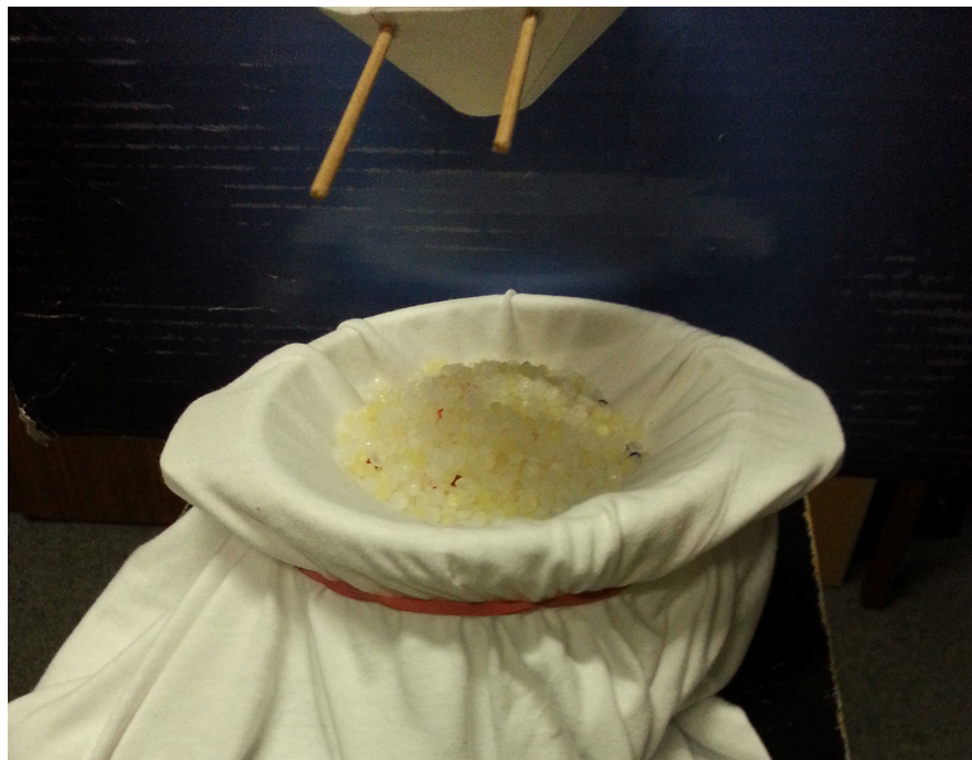
Figure B.5: Void material setup. A cloth is attached to a plastic bowl and the resulting pocket is filled with granular material. This approach is used to obtain sound caused purely by the collision of the grains.
