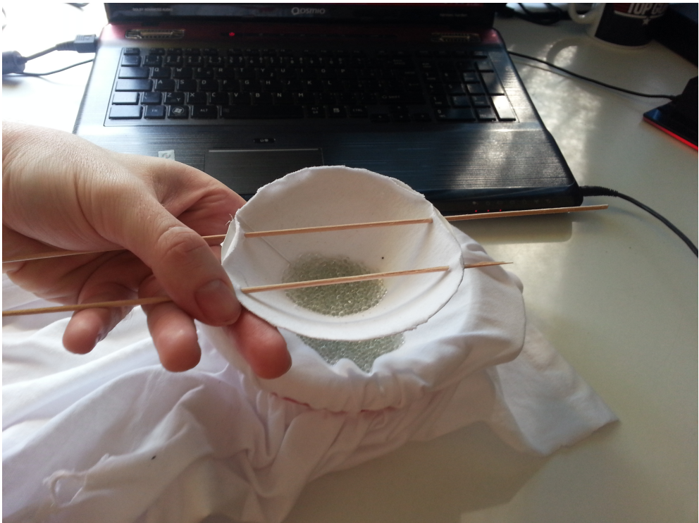
Figure B.3: The funnel used to obtain recordings. Notice the cloth layer glued to the funnel to minimise the sound produced by the interaction of granular material and the funnel.
