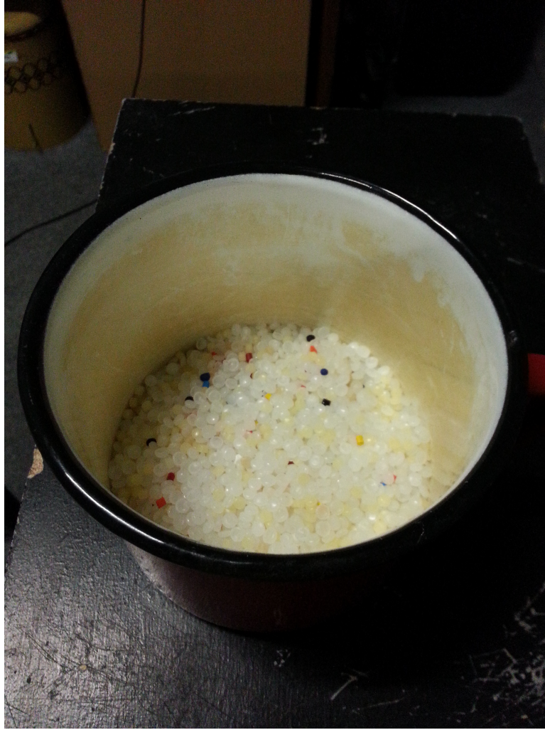
Figure B.6: For each combination of granular material and container, we conducted one recording with a small amount of material already present in the container. This figure show a metal cup filled with plastic, disc-shaped particles of 4mm diameter.
