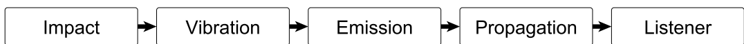
Figure 2.2: The idea of dividing the sound simulation into five separate stages is presented in Thesis [51].
