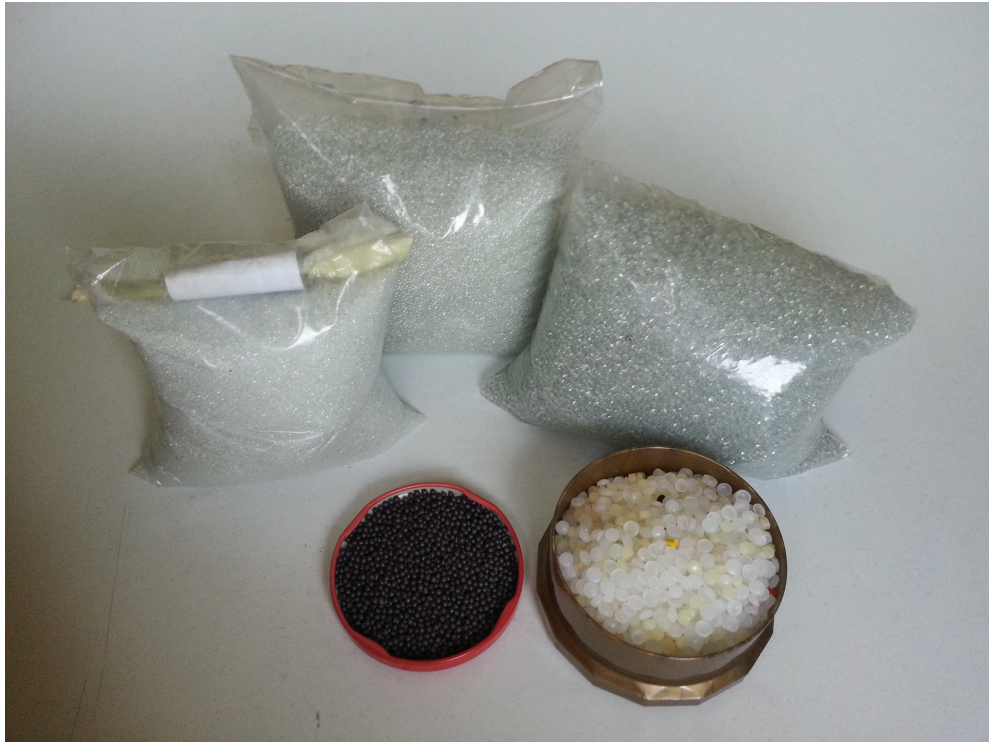
Figure B.1: Granular materials used in the recordings. In the back row, there are three types of glass spheres with different diameters. In the front we can see iron spheres and plastic discs.
