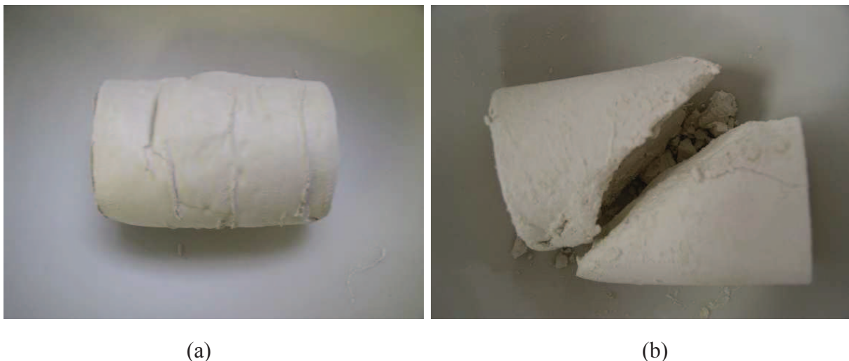
Figure 5.10 Specimens consolidated or compressed up to 100 kPa after rupture: (a) pure kaolin clay; (b) kaolin clay with 4% of Portland cement
