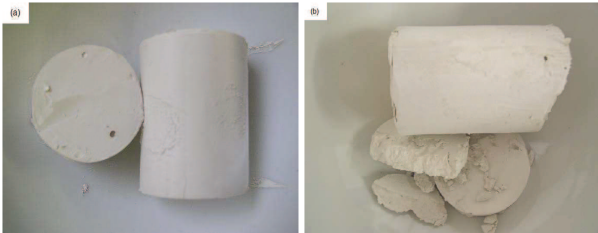
Figure 3.2 Cross section of triaxial specimen after initial consolidation in a rigid cylinder. (a) kaolin clay. (b) cemented kaolin clay.
