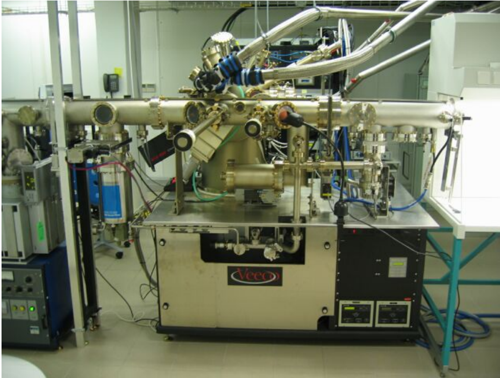
Figure 1.1: The MBE device Veeco in the MBE Laboratory in the Institute of Physics of the ASCR. The picture was taken from http://department.fzu.cz/surfaces/mbe/soubory/veeco/veeco.htm
