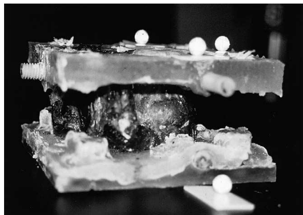
Figure 35 The motion segment for biomechanical testing; the superior and inferior vertebrae were embedded in PMMA, and reflective nylon balls were attached on the PMMA (Tanaka et al., 2001).
