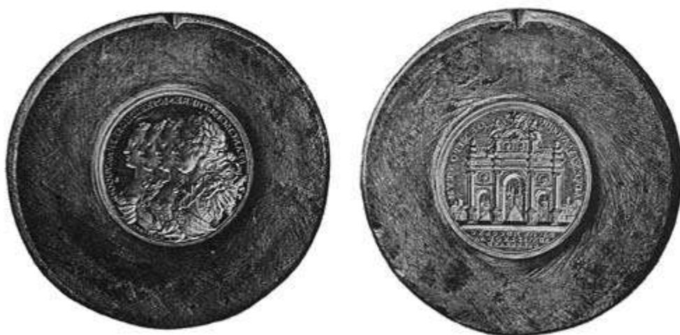
Steel dies of the medal. Each one weights 5 kg
