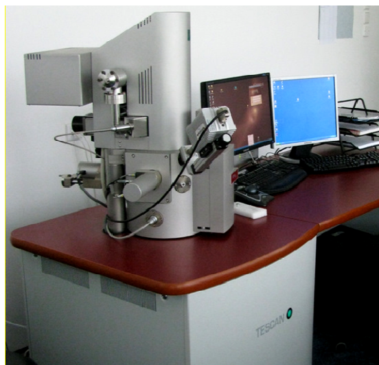
Fig. 5. TESCAN – MIRA scanning electron microscope.
