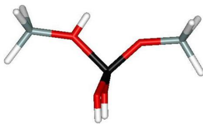
Figure 2.3 3-T cluster model of the Brønsted acid site inside a zeolite
