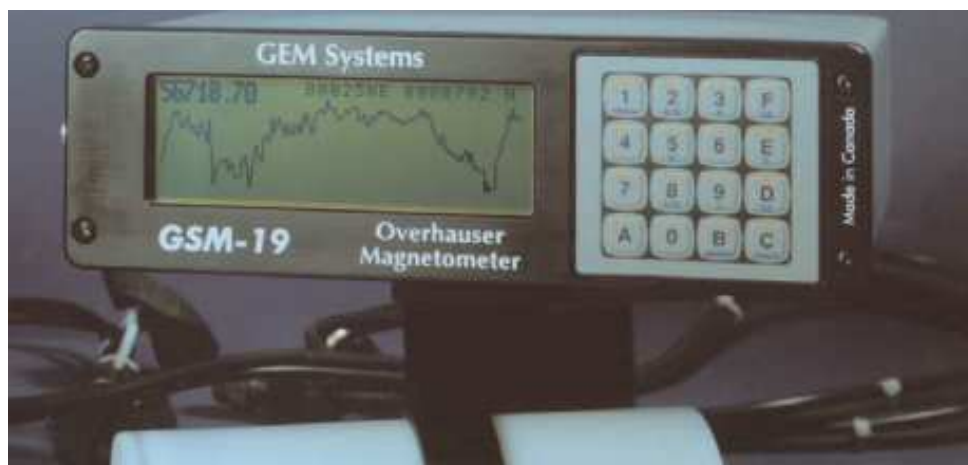
Obr. 24 GSM -19 overhauser magnetometr (GEMsystems, 2013)
