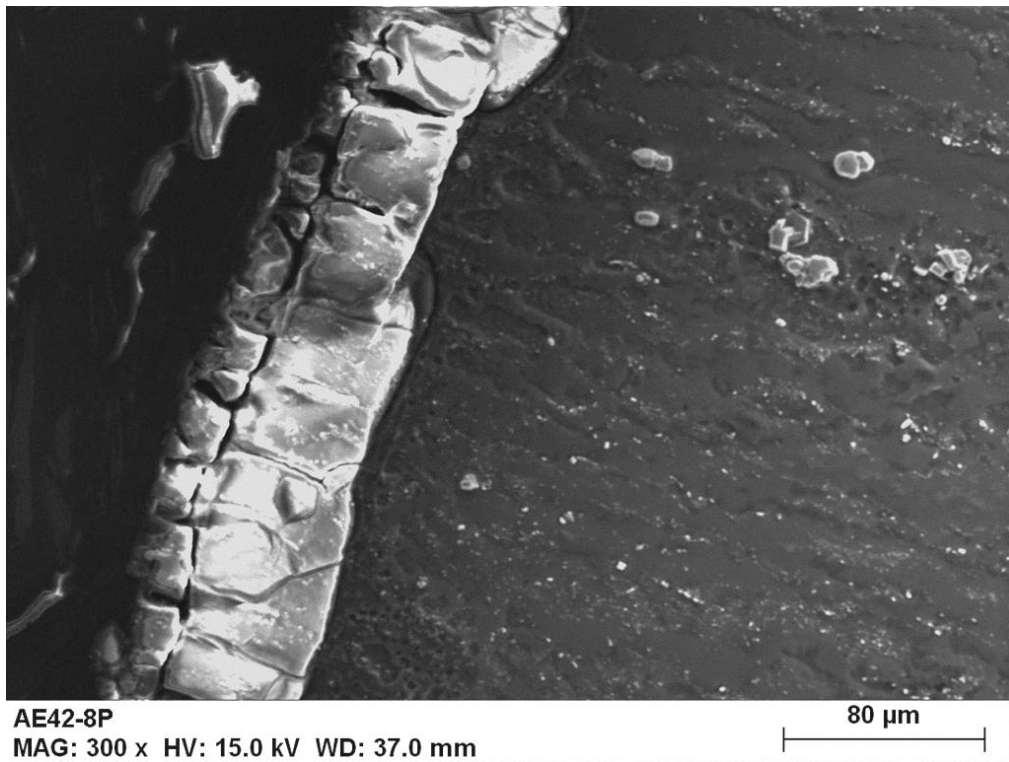
Figure 36: Corrosion layer of the AE42-8P specimen
