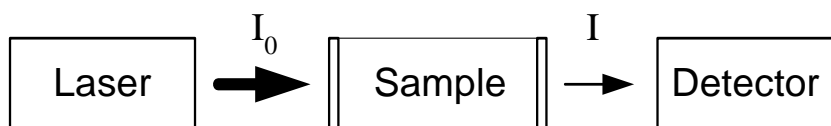
Figure 3.1 Schematic picture of the simplest form of laser absorption spectroscopy measurements. A tunable laser passes through a sample of interest.
