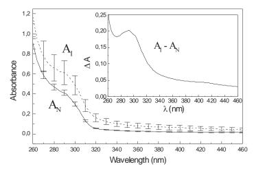
**Figure 4 - B** : Averaged spectra of 4 normal (AN, solid line) and 4 irradiated (AI, dash line) corneal lysates, recorded at dilution 200x, which enabled measurement down to 210 nm. The inset shows again the same data replotted as difference spectrum AI - AN for 210-280 nm.
