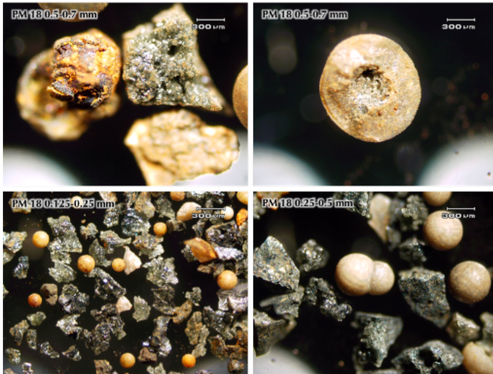
Figure 5.19 Optical micrographs of the debris from PREMIX 18 experiment - small sieving fractions
