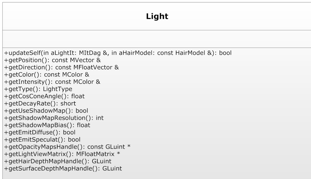
Figure 2.6: Class diagram of Light.
