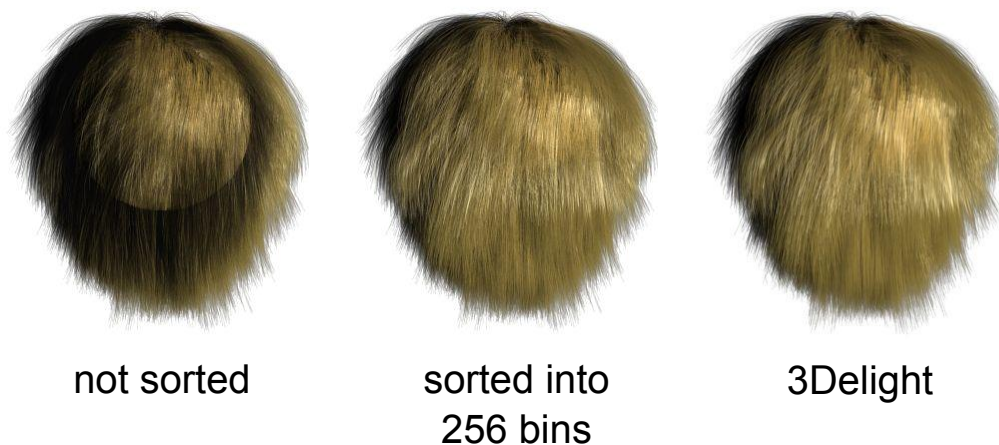
Figure 1.10: Hair geometry rendered without sorting produces very bad results. Approximate line segment sorting into 256 bins shows a result very similar to the reference rendered by 3Delight.
