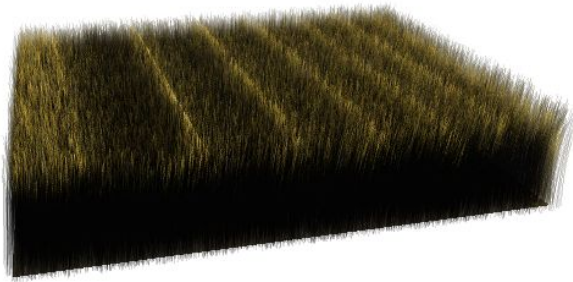
Figure 1.18: Visible artifact when 8 opacity shadow maps are used.
