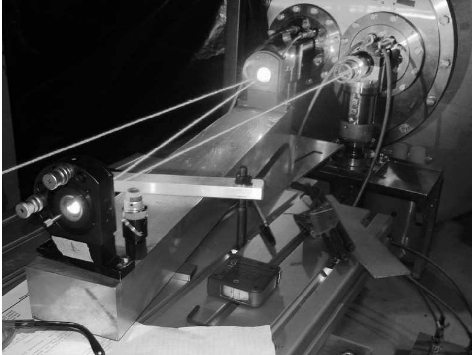
Figure B.22: Laser light at the the entrance of the first magnet of OSQAR. source: < http://osqar.web.cern.ch/osqar/laser.jpg >
