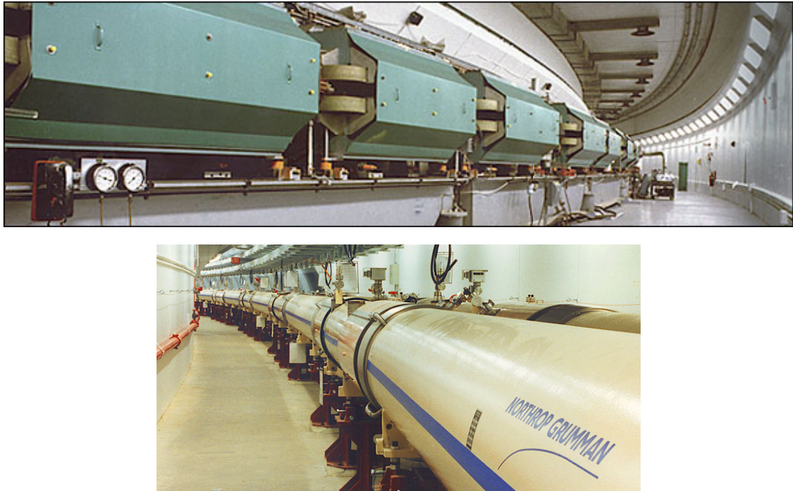
Figure 4.2: top: Magnets of the AGS accelerator. bottom: Inside of the RHIC tunnel.
