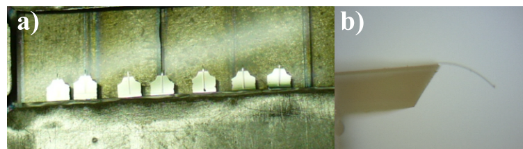
Figure 4.4: Deposition onto cantilevers: a) holder with installed AFM cantilevers; b) a cantilever after deposition is bent due to the intrinsic stress in the deposited \mu\text{c-Si:H} film
